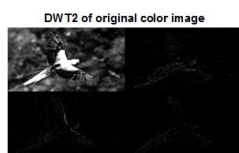
Fig 2: DWT of an Original Image
