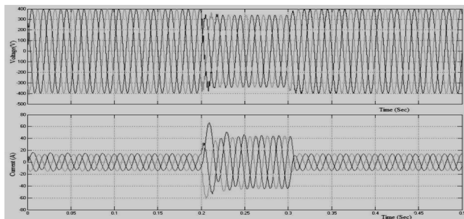
Figure 6. Voltage and current at bus 2 with GUPFC using Fuzzy
