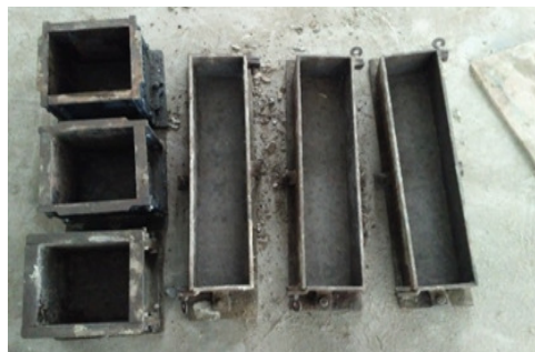
Figure 3. Moulds for casting the concrete
