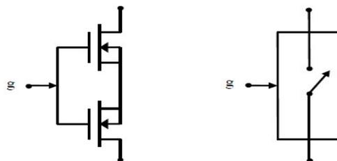
**Figure 6.** Bi-directional Mosfet anti series switch
