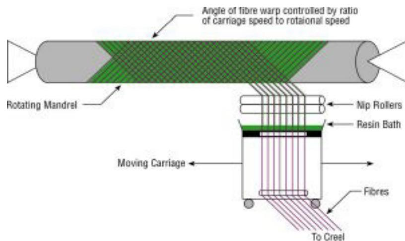
**Figure 1.** Representation of filament winding process
