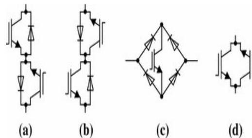
**Figure 5.** Bi-directional switch cell configuration
