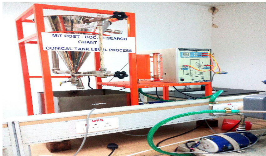
Figure 1. Experimental setup: Conical tank level process
