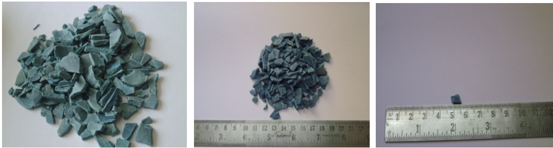
Figure 1. Shape of crushed PVC waste used as Fine Aggregate
