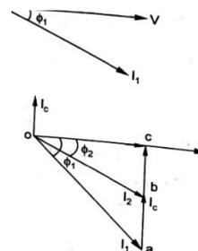
FIG. 1. Power factor improvement based on capacitor bank method.
