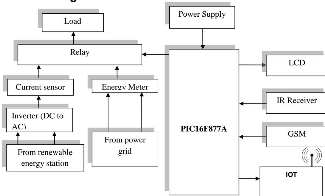
FIG. 2. TOTAL BLOCK DIAGRAM OF IOT APPLICATION ON SMART GRID WITH GRID AND RENEWABLE ENERGIES (DG).
