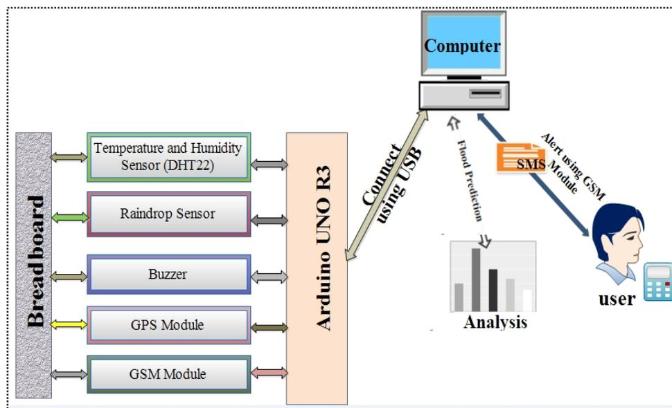
Figure 1. The architecture of the proposed system
