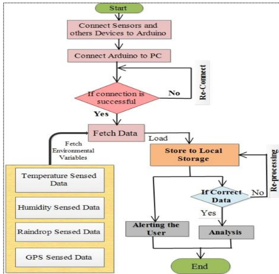
Figure 3- The flowchart of the proposed system
