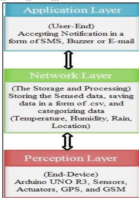
Figure 2 - Layered architecture of the proposed system
