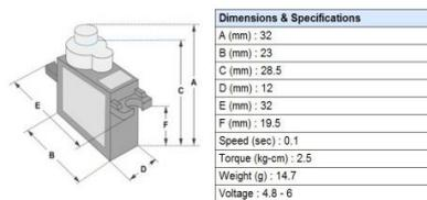
Figure 7: Servo Motor SG90 Data Sheet
