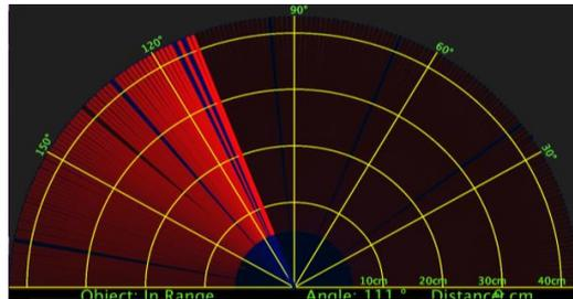
Figure 10: Radar output for obstacle at 9 cm
