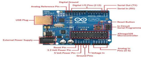
Figure 6: Arduino pin details
