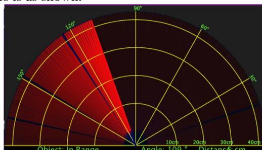
Figure 9: Radar output for obstacle at 5 cm
