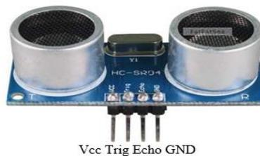
Figure 4: Ultrasonic Sensor HC-SR04
