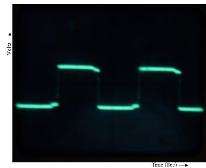
Figure 16: Transformer secondary side AC voltage
