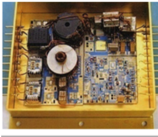
Figure 2: Internal view of 30W HMC DC DC Converter HMC
