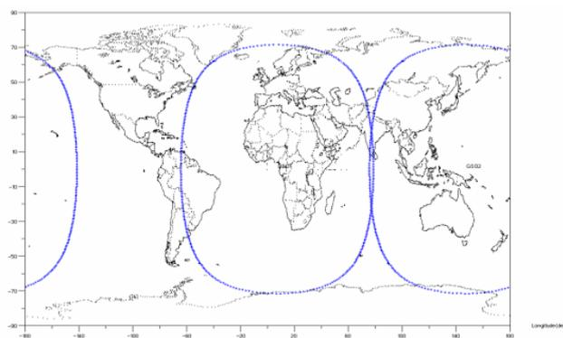
Figure 2: Coverage area of DRS satellites with 1400 separation and 100 elevation contour
