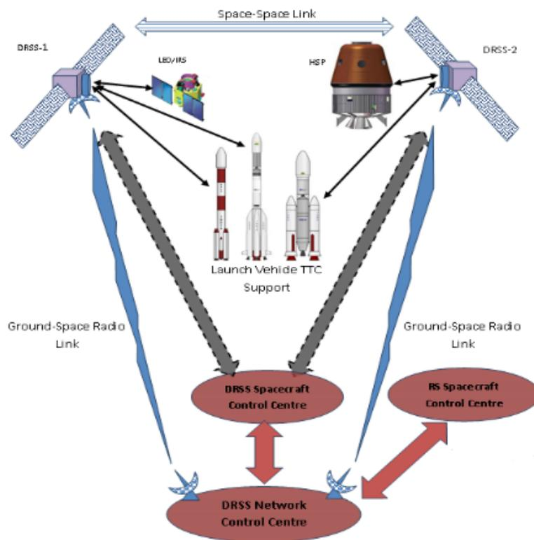
Figure 3: Generic Data Relay Satellite System Architecture
