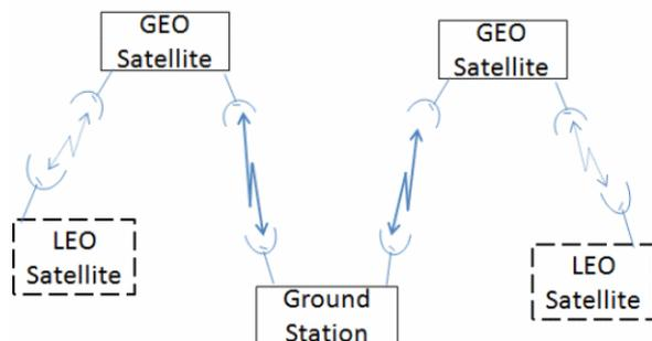
Figure 5: Two IDRSS satellites visible w.r.t ground station located in India
