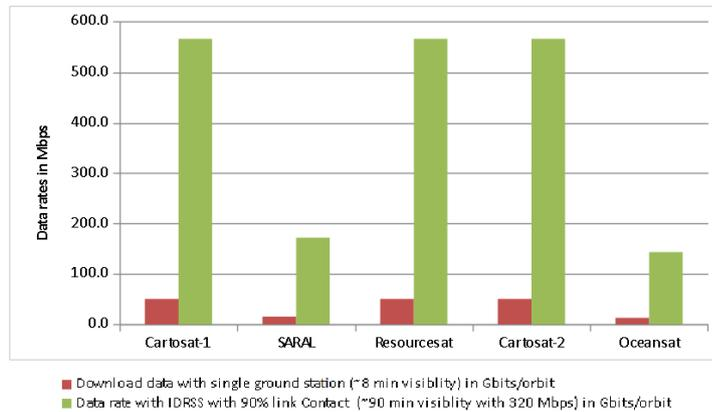
Figure 8: Chart showing increase in data throughput with IDRSS Configuration
