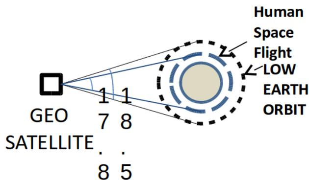
Figure 1: Service area of GEO satellite to HSP flight and LEO satellites
