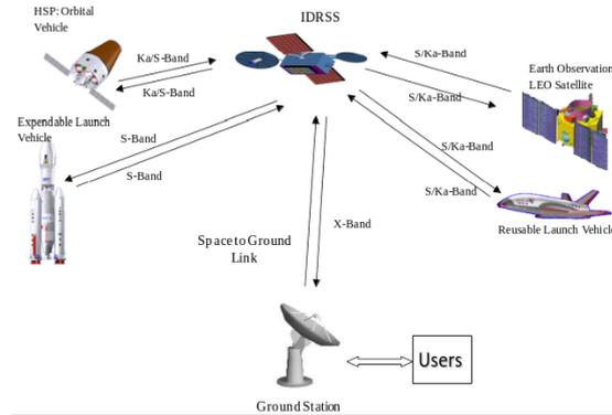
Figure 4: Indian Data Relay Satellite System Architecture
