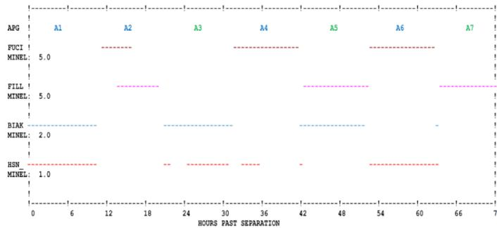
Figure 9: Transfer Orbit visibility Chart of a typical GEO satellite
