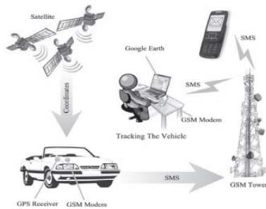
Fig 1: Block diagram of Vehicle Tracking and Anti-theft mechanism [7]
