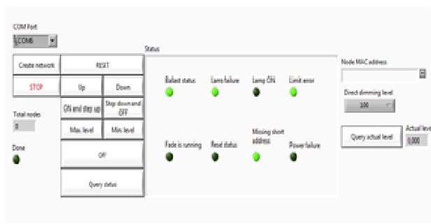
Figure 3. GUI used for DALI lighting control with WSN
