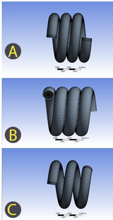
**Figure 3.** the different mesh modelsof tube in tube helical coil heat exchangers A is of pitch 0.045 m B is of pitch 0.07 m C is of pitch 0.09m.
