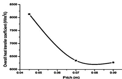
**Figure 8.** showing the graph of the pitch variation and over all heat transfer coefficient of tube in tube helical coil heat exchanger.
