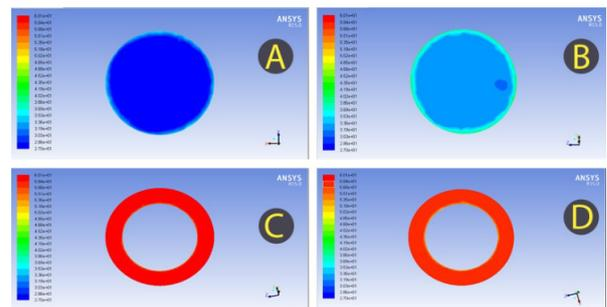
pitch 0.07 A is cold water inlet B is the cold water outlet and C is the hot water inlet and D is the hot water outlet
