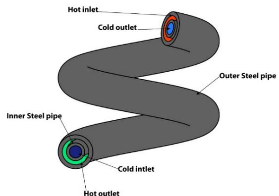
**Figure 2.** boundary conditions of the numerical simulation of the double pipe helical heat exchanger
