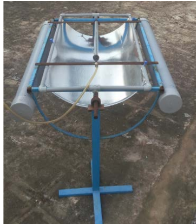
Figure 1: Photograph of the Compact Parabolic Trough Collector
