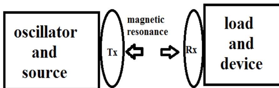
Fig. 1: Block Diagram of Witricity
