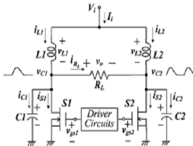
Fig. 2: Basic Push Pull Class E Power Amplifier
