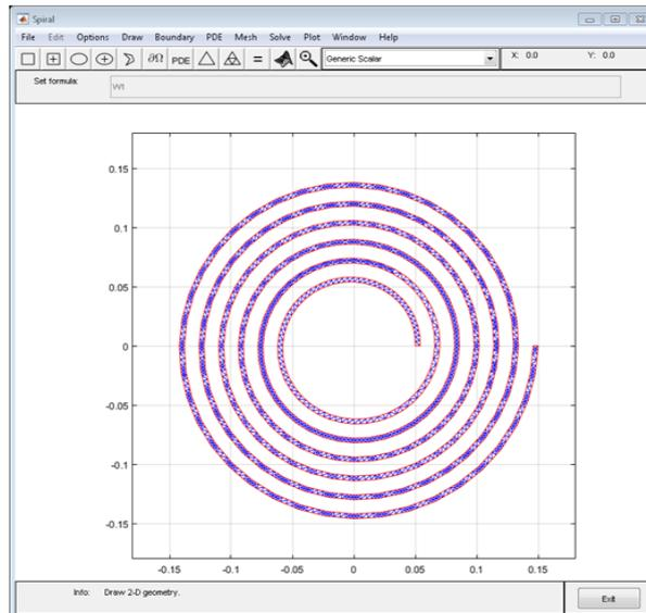
Fig. 5: Spiral Coil Using Pdetool
