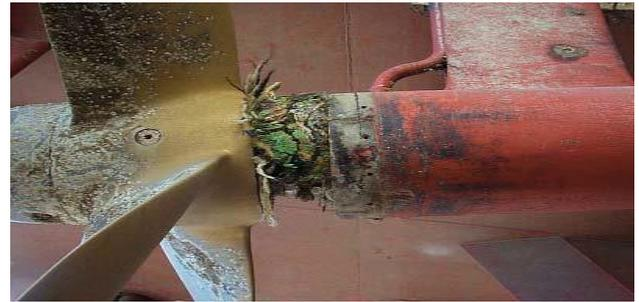
**Figure 3.** Fishing net or rope caught on ships rotating shaft.
