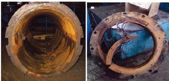
**Figure 4.** Completely damaged oil-lubricated slide bearing and sealing of ship propeller shaft [4]
