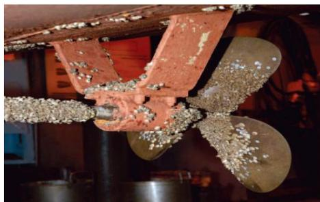
**Figure 5.** Cantilever open bearing of yacht's propeller shaft [4]
