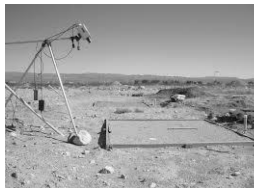
Figure 2. FLIR thermal infrared camera to checkTech land mine detection test facility
