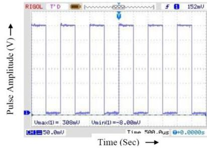
Fig. 6. Gate Pulse for MOSFET Switches (Upper)
