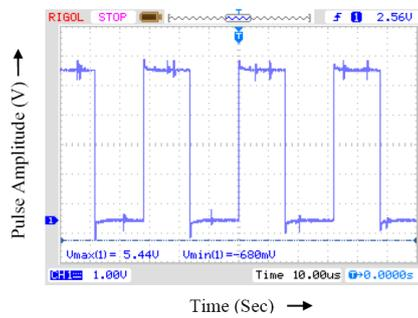
Fig. 7. Gate Pulse for MOSFET Switches (Lower)
