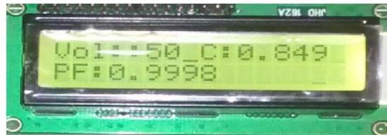
Fig. 10. Input Power Factor Display- Loading Condition
