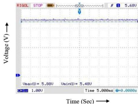
Fig. 5. Output Voltage of Cuk Converter
