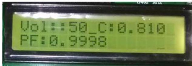
Fig. 9. Input Power Factor Display- No Load Condition
