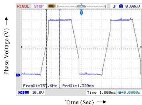
Fig. 8. Input Voltage Waveform to Motor
