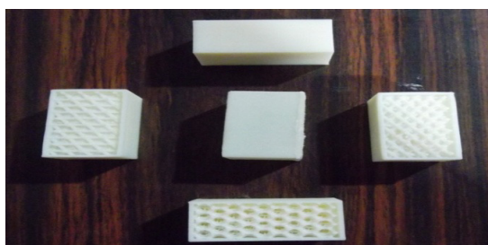
Figure 12. Internal structures after post curing process
