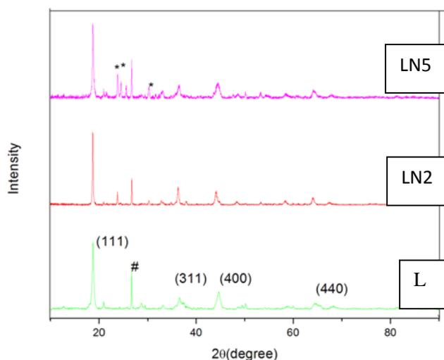
Figure 1: XRD spectrum of LP)  $\text{Li}_2\text{Mn}_2\text{O}_9$  LN2)  $\text{Li}_2\text{Mn}_{3.75}\text{Nb}_{0.25}\text{O}_9$  LM5)  $\text{Li}_2\text{Mn}_{3.5}\text{Nb}_{0.5}\text{O}_9$
