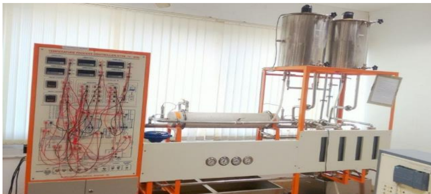
Figure.1 Heat exchanger experimental setup
