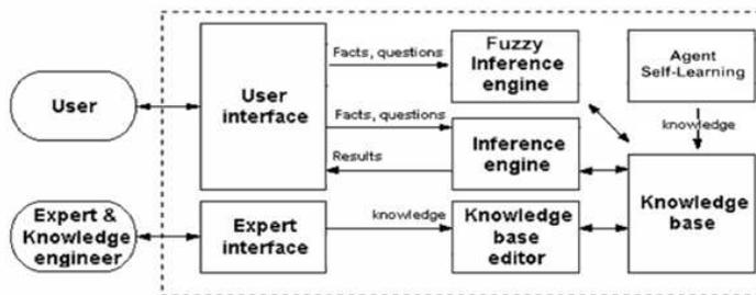
Figure 4: System Component Integration of Proposed Fault Troubleshooter
