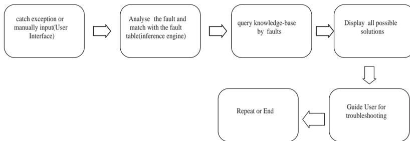
Figure 6: Program Flowchart for Proposed Model
