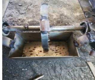
Figure 1: Seed sowing disc and hopper
