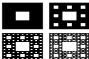
Fig.4 Sierpinski Carpet Fractal Antenna
