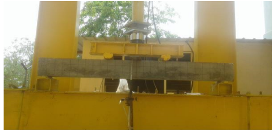
Figure 8: Arrangement of Beam Specimen on loading frame for testing
