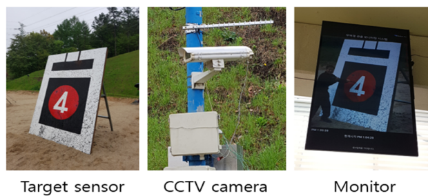
Figure 3: Target system configuration status
