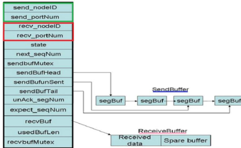
Figure 1: TCB with send buffer and receive buffer
