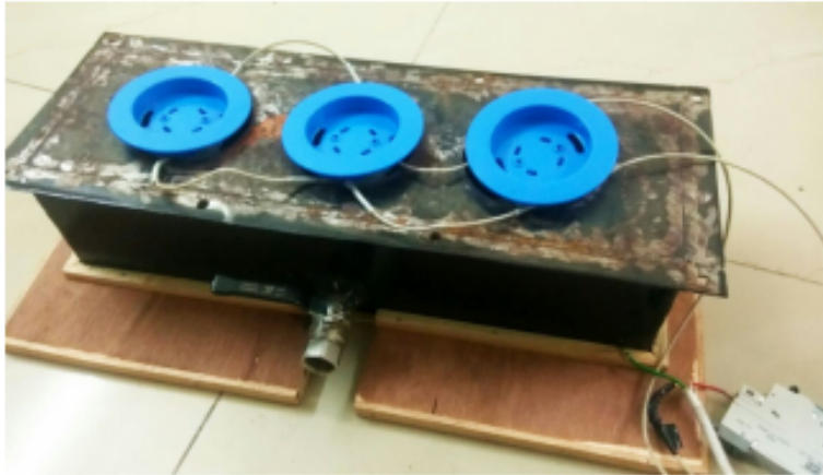
Figure 4 steam unit with a heating unit
