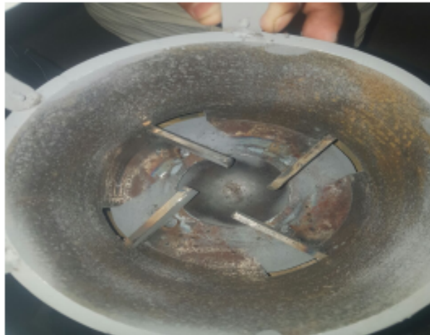
Figure 6 Top view of the vortex chamber.
