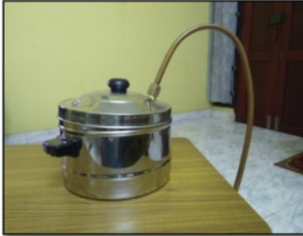
Figure 8 Image of the Pressure Vessel and the Copper Tube for pyrolysis
