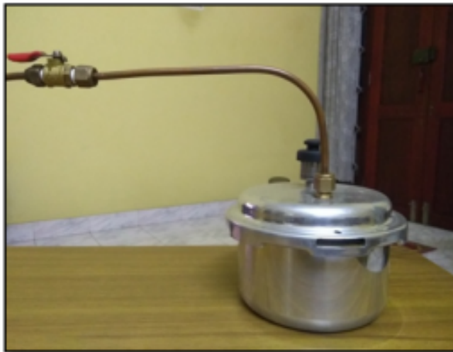
Figure 9 Image of the Pressure Vessel and the Copper Tube for steam generation
