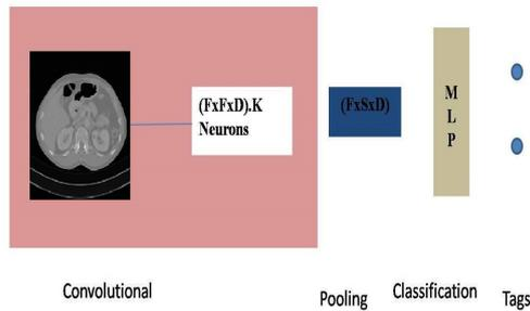
Fig. 5. Automatic Feature Extraction based CNN Classifier
