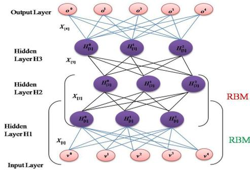
Fig. 2. A typical stack of Restricted-Boltzmann Machine
