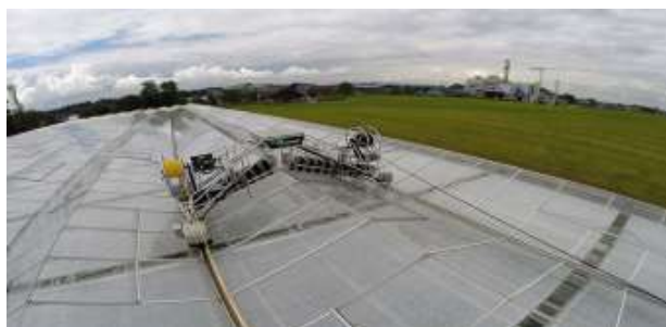
Fig.3. Automatic Greenhouse Roof Cleaner
