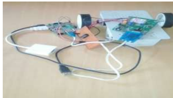
Fig.5. Experimental Implementation of Didactic Robot Model using Raspberry-pi3
