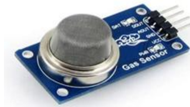
Fig .3: Gas Sensor.
