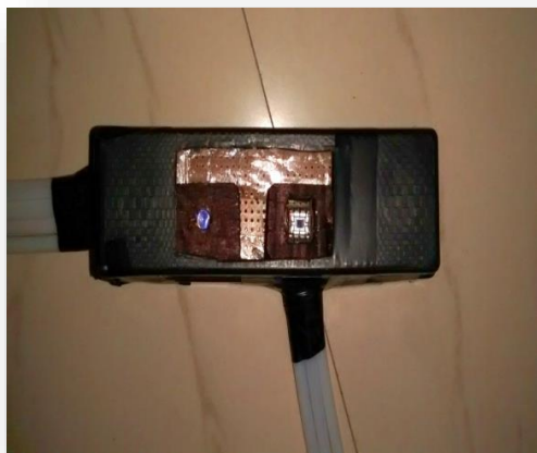
Fig 1.: Sensor unit with led and detector at an interoptode distance of 3cm
