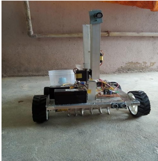
Figure 4.5.Obstacle detection and obstacle clearance
