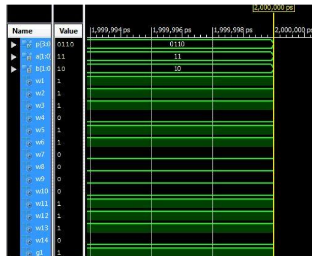
Fig.10 (c) Simulation result of Reversible Fault Tolerant 2*2 Vedic Multiplier
