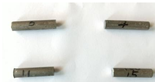
Fig. 1: Shows the Sample Specimen of Diameter 6 mm and Length 30 mm
