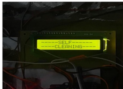
7.)"SELF CLEANING" when automatic mode is switched on.
