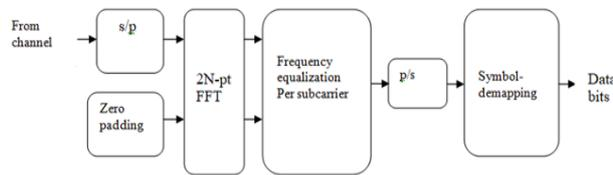
Fig. 4. Block diagram of UFMC-Receiver
