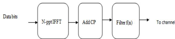
Fig. 5. Block diagram of F-OFDM-transmitter
