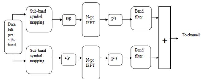
Fig. 3. Block diagram of UFMC-Transmitter
