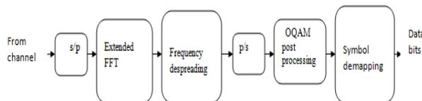
Fig. 2. Block diagram of FBMC-Receiver
