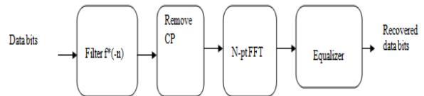
Fig. 6. Block diagram of F-OFDM-Receiver
