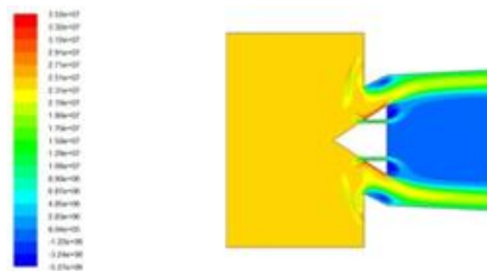
Fig 4.4: Total Pressure Contour (M = 3) with holes in spike
