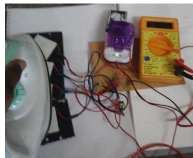
Fig. 7 : charging the sample mobile battery using TEG by waste heat
