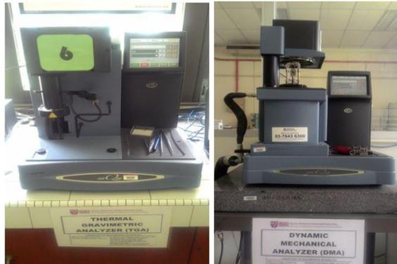
Figure 1. Characterization equipments (TGA and DMA)
