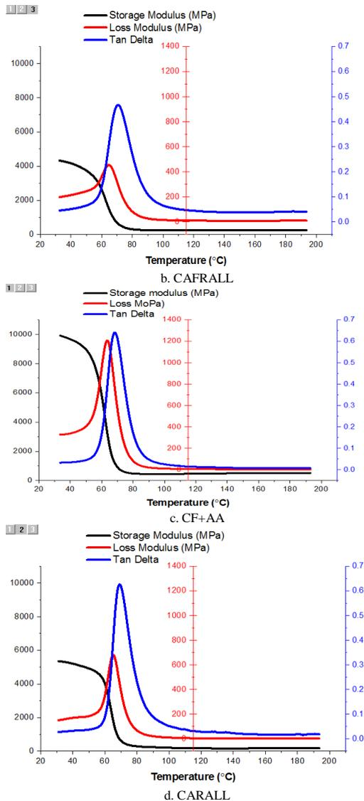
Figure 4. Dynamic mechanical analysis for the Composites
