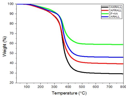
Figure 2. Thermogravimetric curves for the composites
