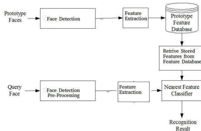
Fig. 4. Feature Extraction in face recognition
