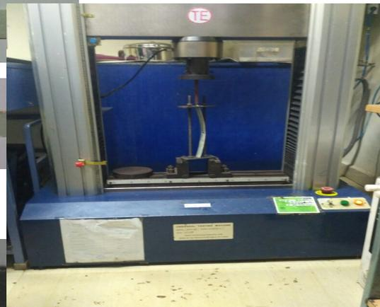
Fig 4 Buckling setup in UTM machine
