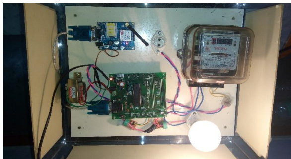
Fig. 1.5 When Unauthorisedload is Connected
