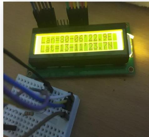
Fig : Output of GPS as displayed in LCD.
