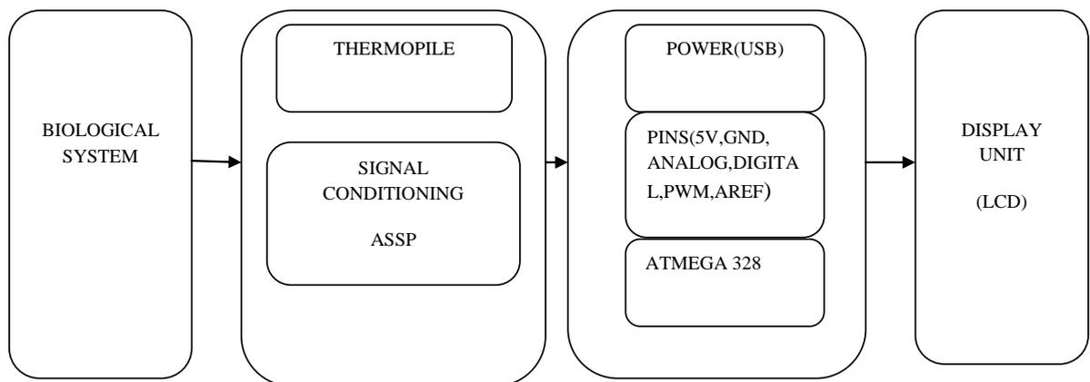
**FIGURE 4: BLOCK DIAGRAM OF THE PROPOSED SYSTEM**
