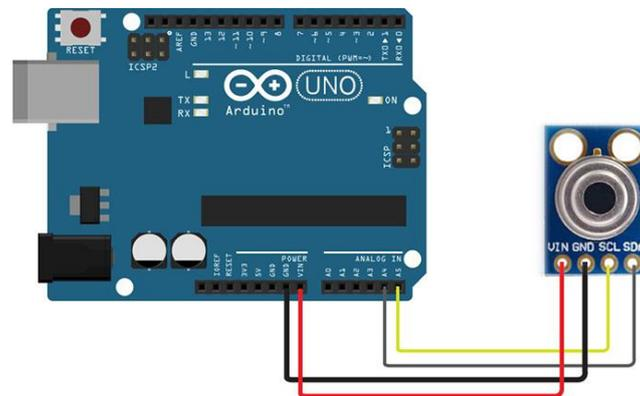
**FIGURE 7: INTEGRATION OF MLX90614 IR THERMAL SENSOR WITH ARDUINO UNO (ATMEGA 328) BOARD**
