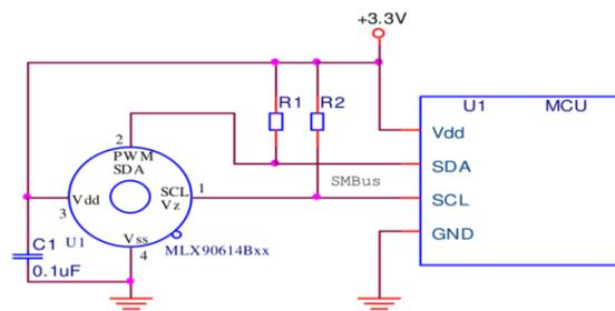
**FIGURE 5: CIRCUIT DIAGRAM OF INFRARED THERMAL SENSOR (Mlx90614)**
