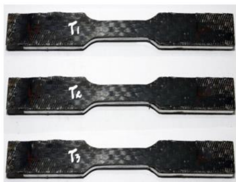
Figure 3: Fractured specimen after the testing
