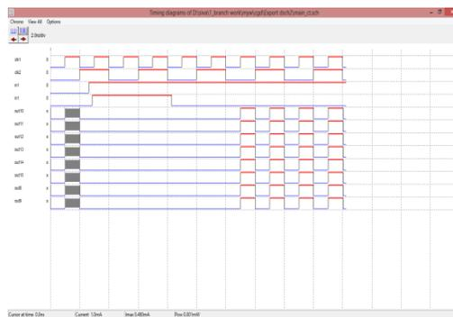
Fig 4: output of 3-d gated clock tree
